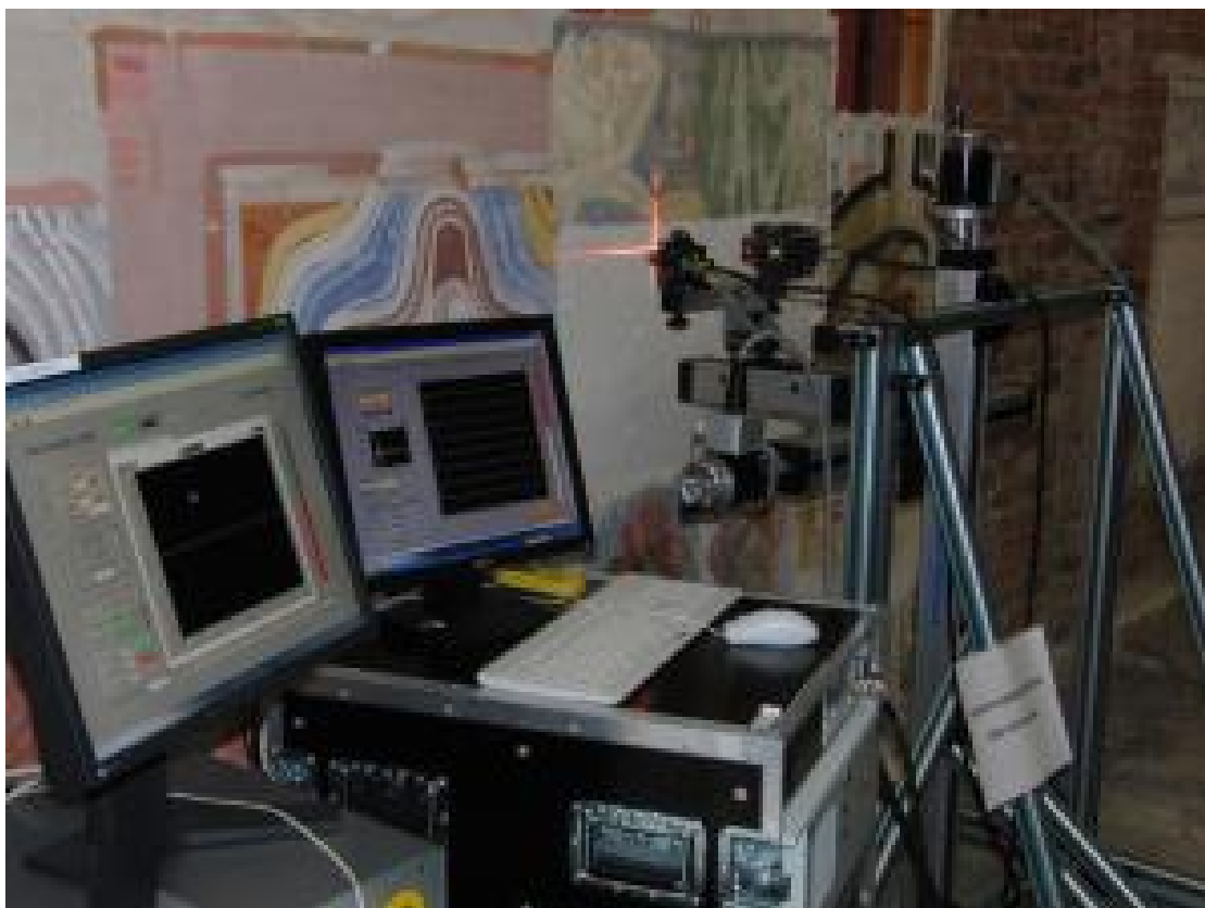
The mobile scanner at work on a test wall. A software system reveals the structure of the concealed paintings. (Credit: Copyright Fraunhofer IWS)
